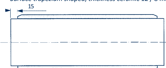
STS 4000 ceramic drum lagging, mounted directly on a cylindrical drum. Maximum thickness ceramic 15 mm.
