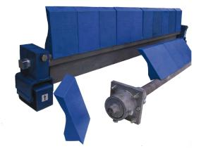
The conveyor belt scraper is standard provided with bluecoloured polyurethane segments: 150 mm segment width, galvanised construction, including tension elements. The installed width is variable. Loose segments can be delivered and are easily exchanged.
